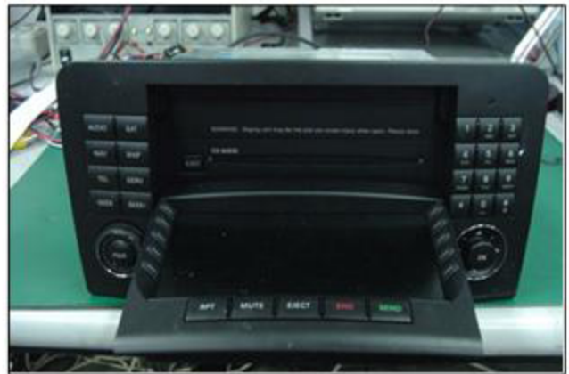
STEP 7: Press the eject button to keep face open and then disconnect power.
