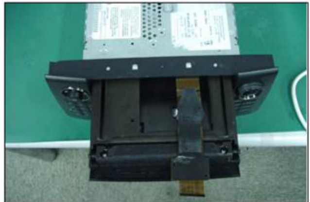
STEP 9: Disconnect the ribbon cable from the display section of the navigation unit.
