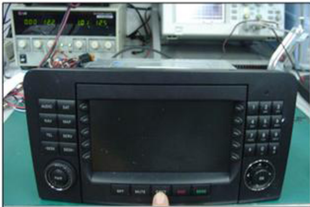
STEP 6: Power up unit on bench.
