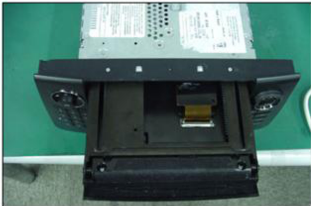
STEP 8: Turn unit upside down to expose the ribbon cable underneath the face of the unit.
