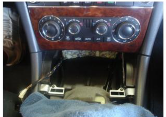
STEP 4: Cover shift knob and base trim in a towel to protect from any damage.
