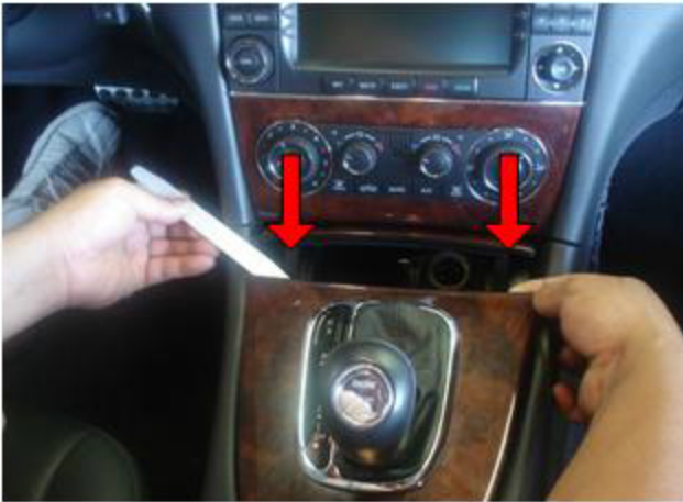
STEP 1: Using a plastic pry tool, pry up on wooden trim around the shifter base to release (2) plastic snaps.
