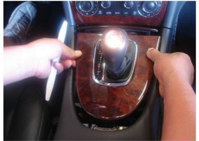
STEP 2: Release the trim base and place shifter in lowest gear to move base out of the way.
