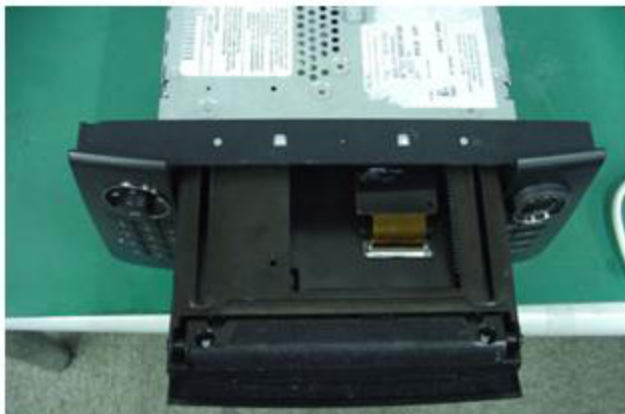
STEP 13: Turn unit upside down to expose the ribbon cable underneath the face of the unit.
