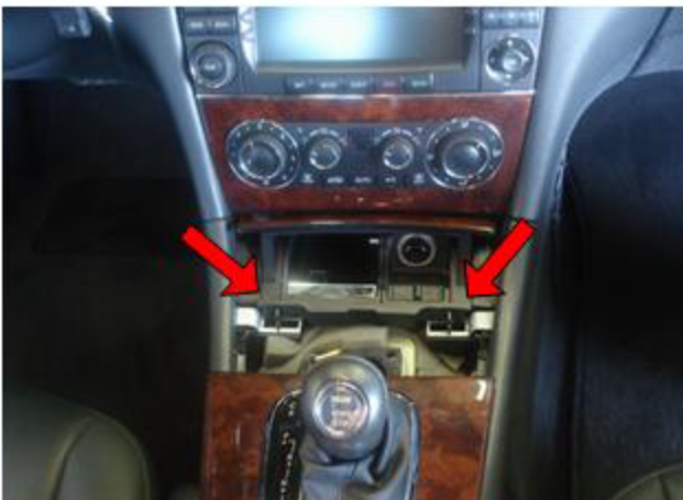
STEP 3: Unclip ashtray and cigarette lighter, disconnect wires and completely pull piece out of center console.
