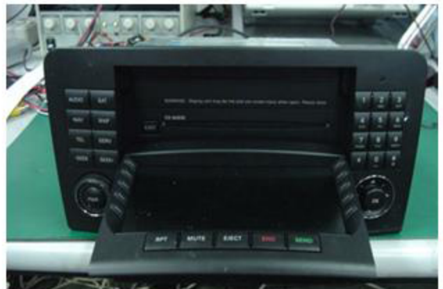
STEP 12: Press the eject button to keep face open.
