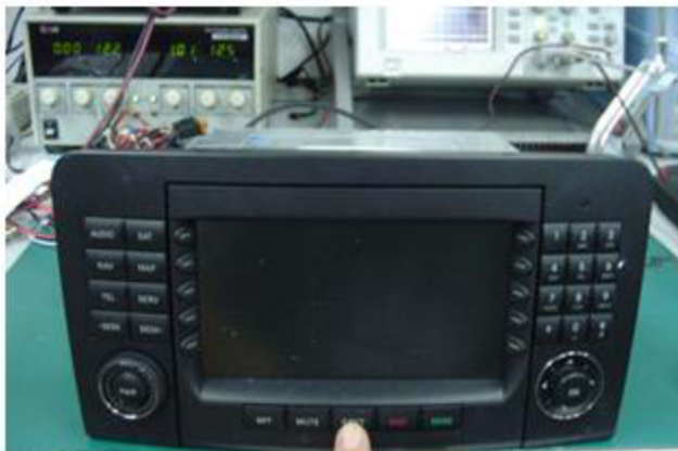
STEP 11: Power up unit on bench.
