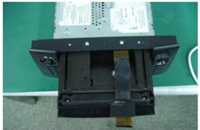
STEP 14: Disconnect the ribbon cable from the display section of the navigation unit.
