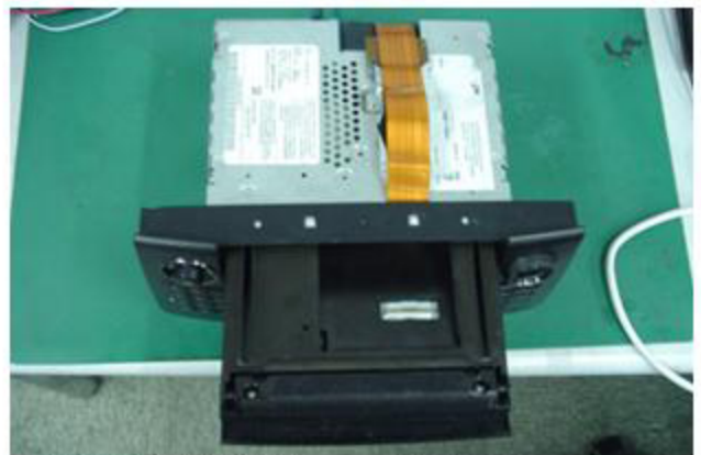
STEP 16: Pull ribbon cable back and leave exposed.
