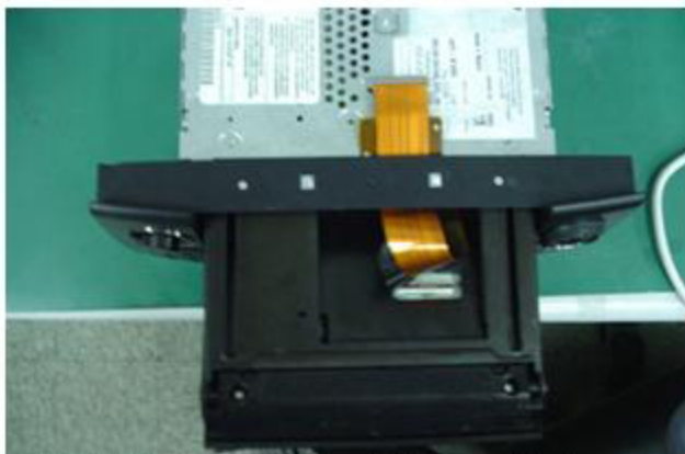
STEP 15: Loosen the ribbon cable from the chassis.
